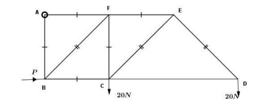
The above framework consists of nine smoothly jointed light rods, smoothly hinged to a fixed point at A, kept in equilibrium by a horizontal force P at B and loaded with 20 *W* each at C and D.
