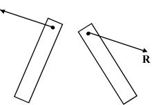
X, Y are the horizontal and vertical components of R. R is the resultant of X and Y, and passes through the pinjoint.  $\checkmark$
