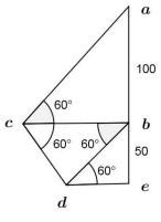
In the above diagram regions are named starting from C and the stress diagram 100 is drawn as follows.
