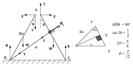
For the equilibrium of the ring  $R_1 = T$  and  $R_1$  is perpendicular to AC, so T is perpendicular to AC
