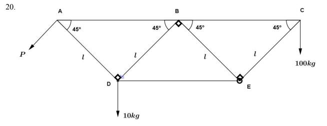
The above framework is made by seven light rods AB, BC, AD, BD, BE, CE and DE where  $AD = BD = BE = CE = \ell$ . The frame is hinged at E, kept in equilibrium by a force P applied at A, with loads 100 kg at C and 10 kg at D.
