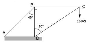
The given figure shows a crane composed of four freely jointed rods AB, BC, CD and BD. The rod BC is horizontal while the rod BD is vertical. The crane is fixed to the horizontal ground at A and D and there is a load of 1 000 N hanging at C. Use Bow's notation to find the forces in the rods, distinguishing between tensions and thrusts.
