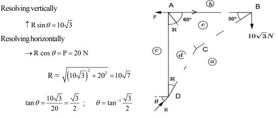
Since the system is in equilibrium under three forces the reaction R should also pass through B. Start from joint B in the anticlockwise direction.
