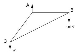
In the given figure, ABC is a triangular framework consisting of three smoothly jointed light rods AB, BC, CA, where AB = ACand  $BAC=120^{\circ}$ . The framework is in a vertical plane with AB horizontal. It is supported at A by a smooth peg and carries loads 100 N at B and WN at C. Draw a stress diagram using Bow's notation and from it, calculate the stresses in the rods, distinguishing between tensions and thrusts and also find the value of W.
