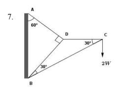
The figure shows a framework consisting freely jointed four light bars AD, BD, BC and CD. It is hinged freely to a vertical wall at A and B. C carries a load of 2W. By using stress diagram find the reactions at A and B. Hence find the stresses in the rods distinguishing tensions and thrusts.
