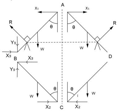
The system is symmetrical about AC. Therefore, the vertical components of the reaction at A and C are zero.
