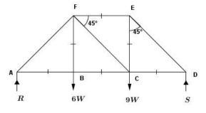
9. A freely jointed framework consisting of five light rods is shown in the figure. Joint B carries a load of 900N. The framework is in equilibrium such as AD is vertical by means of forces P and (P, Q) acting on A and D respectively (P is horizontal and Q is vertical). Find the magnitudes of forces P and Q. Draw the stress diagram using Bow's notation and find the stress in each rod, distinguishing tensions and thrusts.
