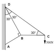
At joint C one force is known and two forces unknown. Draw the stress diagram starting from joint C.
