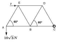
The given figure shows a framework consisting of seven light rods AB, BC, CD, DE, EA, EB and BD smoothly jointed at their extremities. The frame smoothly jointed at C and carries a
