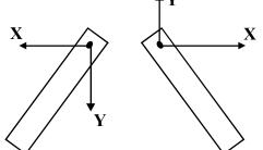
The light pin is assumed to be a small smooth pin of circular rim, joins the rod by passing through the rods. As the pin is smooth the reaction on contact is perpendicular to it and for rods. Since the pin is in equilibirium under these two forces, they are equal opposite in direction and have the sameline of action. Therefore the reaction on each rod is equal and opposite and have the same line of action an each joints.
