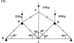
The given figure represents a framework of light bars loaded at joints B, F, D as indicated. The bars AC and CE are horizontal and each equal to 10 m and CF = 8 m. Also the lengths AB = BC = CD = DE and BF = FD. The frame rests on two smooth pegs at A and E. Calculate the reactions at A and E assuming that they are vertical. Draw a stress and find the stresses in the rods distinguishing between tensions and thrusts.
