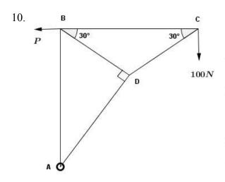
Five light rods are freely jointed to form the framework shown in the above figure. The framework is in equilibrium in a vertical plane with joint A freely hinged to a fixed point. AB is vertical, BC is horizontal,  $A\hat{D}B = 90^{\circ}$  and  $D\hat{B}C = D\hat{C}B = 30^{\circ}$ . A load of 100 N hangs at C and a horizontal force P acts at B in the direction of CB.
