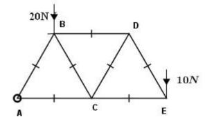
The above figure shows a framework made by seven light rods. The frame is hinged at A to a fixed point and kept in position by a horizontal force P at B. Draw a stress diagram using Bow's notation and find the stress in each rod distinguishing between tensions and thrusts.
