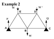
ABCDE is a frame made of seven equal light rods and rests on two pegs at A and C. It carries W at E, B and W' at D. The external forces P, Q will be vertical.
